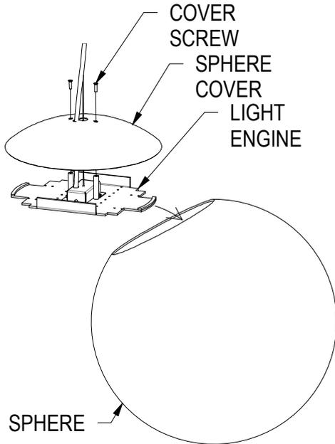
**NOTE:** If Light Engine is shipped separate from Sphere, assembly fixture as shown. Secure Sphere Cover with Screws.
